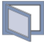
Side hung casement inward opening
