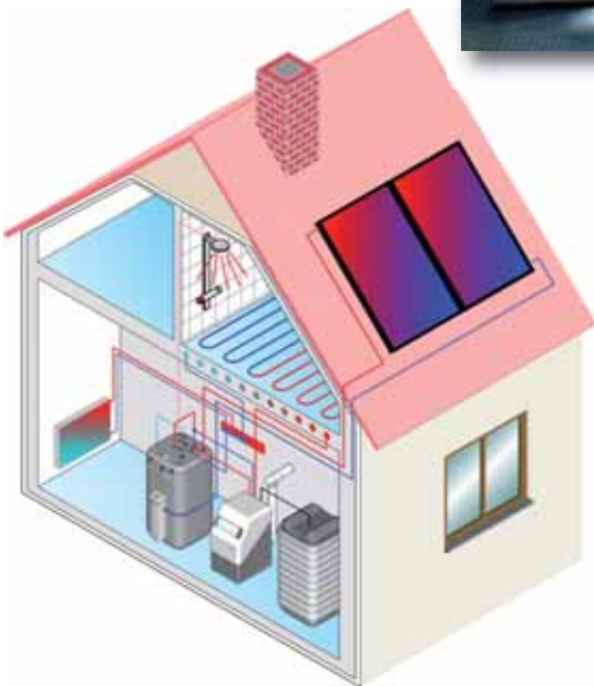
Caldera Gasoil + Solar
